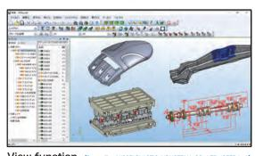
Because synchronized function of hierarchy and a parts, operation is enabled comfortably even for big assembly data. Furthermore, PMI and point of view are supported for JT data.
